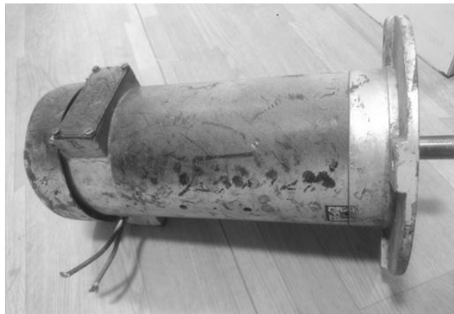
Fig 3:PMDC motor (1HP, 24V, 38A, 1500 rpm)
