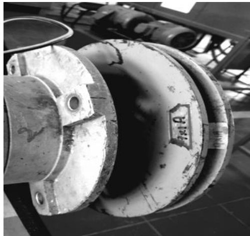
Fig 4: Rotational load-Flywheel(22.9cm diameter, 12kg)
